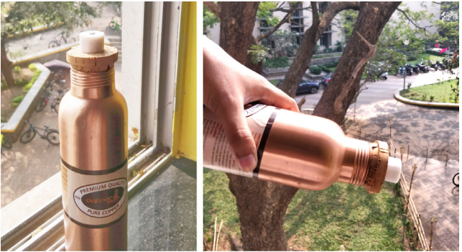
proof of concept rig to show that a cork top works as a watertight closure
